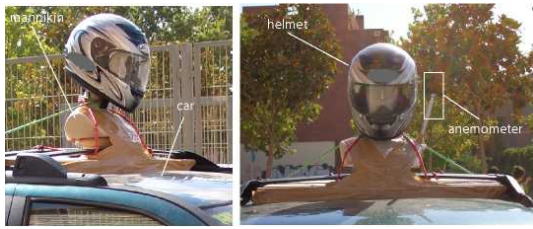
Figure 1: Setup for the freeway experiment: mannikin and helmet with microphones and anemometer, all located in the car's roof.
